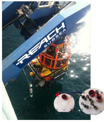
The Orion sensor array only needs to be brought in the approximate vicinity of the utility line to calculate a relative position. Using at least two 3D magnetic field sensors, a triaxal accelerometer and digital compass, Orion identifies the horizontal offset, vertical depth, tone current strength and yaw
