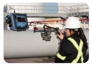
A detector, the GLIDER™ dedicated probes and hed for CFRP flat panel and on. **pection** The OmniScan PA system with the HydroFORM scanner is designed to offer the best inspection solution for the detection of wall-thickness reductions resulting from corrosion, abrasion, and erosion. For this application, phased array ultrasound technology offers superior inspection speed, data point density, and detection.
