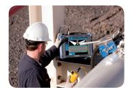
A complete inspection of pressure vessel welds can be performed manually, or in a single scan using an OmniScan and a scanner for a turnkey solution. Inspection results are available immediately, enabling you to detect problems with welding equipment and fix them right away.
