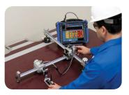
Olympus offers complete solutions for the inspection of carbon-fiberreinforced polymer structures. These solutions are based on the OmniScan flaw detector, the GLIDER<sup>™</sup> scanner, and dedicated probes and wedges designed for CFRP flat panel and radius inspection.
