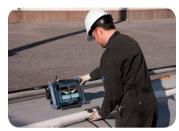
When coupled with the COBRA manual scanner, the OmniScan flaw detector is capable of inspecting pipes ranging from 0.84 inch OD to 4.5 inch OD. With its very slim design, this manual scanner is able to inspect pipes in areas with limited access.
