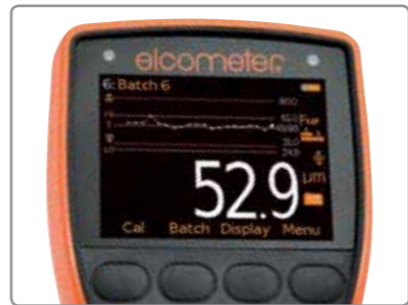
On-screen trend graph displaying last 20 measurement values
