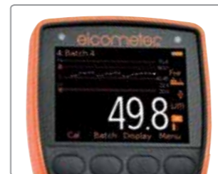
The Run Chart displays each individual reading allowing the user to identify any significant trends
