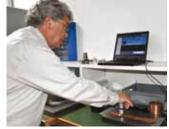
Equostat 3 probe connected to PC
