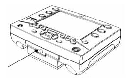
Fig 1.1 - Position of Tripod Mount
