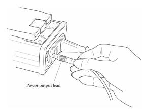
Fig 5.5 Connecting the Power Output Lead to the Charger
