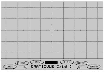
Fig 2.6 GRID 1 - A square graticule marking - X and Y positions marked at 20%
