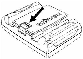
Fig 5.1 Location of the Battery Release Catch
