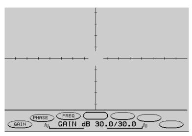
Figure 2.2 - Locator 2s operating screen
