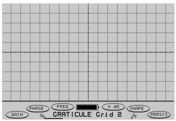
Fig 2.7 GRID 2 – A square graticule with X and Y positions marked at 10%
