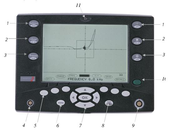
Figure 2.1 – Locator 2s Front Panel Controls
