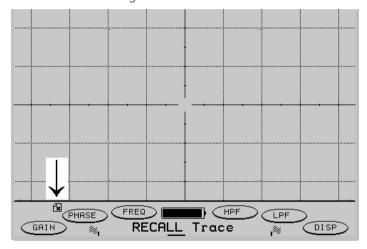
Fig 3.4 Recalled Trace with flashing reference trace icon indicated
