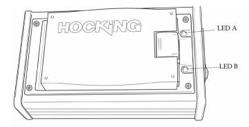
Fig 5.2 Location of the Battery Charger Indication LEDs
