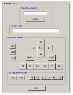
Fig 6.11 Remote Control Panel
