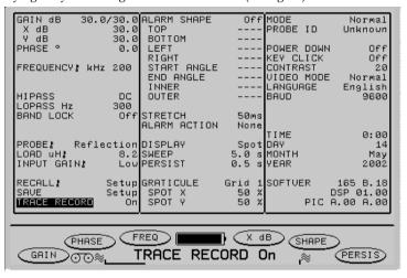
Fig 3.7 Trace Record Menu screen showing Locked items
