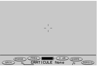
Fig 2.5 NONE – A clear graticule with cross-hairs for identifying the origin
