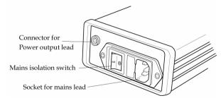
Fig 5.3 Location of the Battery Charger Connections
