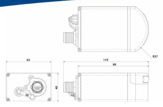
Drawing shown with Seacon connector. All dimensions are in mm, not to scale
